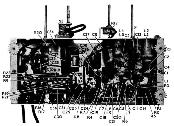
NOTE: The I.F. transformer primary cores are adjusted from underneath the chassis.
